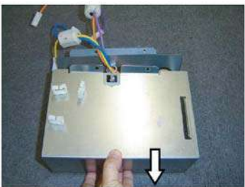
Remove the CONDENSER COVER by sliding toward.
