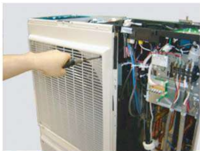
Remove the 4 mounting screws.
