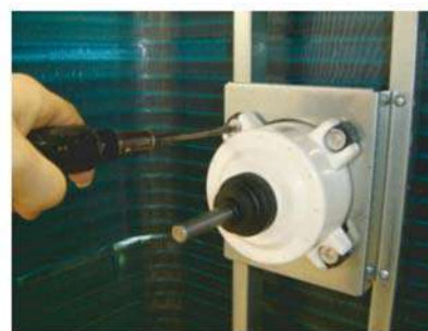
Remove the 4 mounting screws. Remove the FAN MOTOR.
