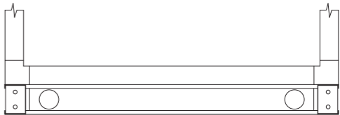
SECTION VIEW The baseframe is flush with the panel.
