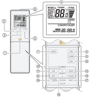
①Start/Stop button 2 "10 °C HEAT" button 3 "TEMP. ( $\land \lor$ )" button ④Remote controller display 5"ECONOMY" button **(6)**Signal transmitter ⑦"MODE" button (8)"FAN" button (9)"SWING" button 10"SET (Vertical airflow)" button 10"ON" timer button 12"OFF" timer button 13"SLEEP" button (4) "CANCEL" button (5)"SELECT (△▽)" button 16"CLOCK ADJUST" button 17 "RESET" button\* 18"TEST RUN" button\*
