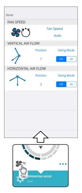
By selecting each item as shown on the screen, you can set the Fan speed and airflow direction. For detailed information on each setting, see the operating manual of the air conditioner.
