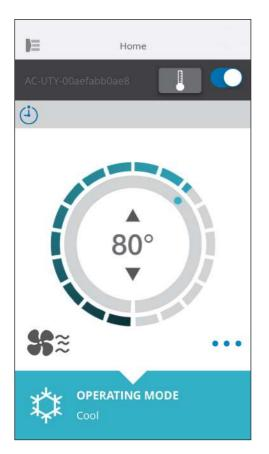
By tapping ▲▼ icons or by tracing the outer rim (circle) of the current temperature, you can set the temperature of your choice.
