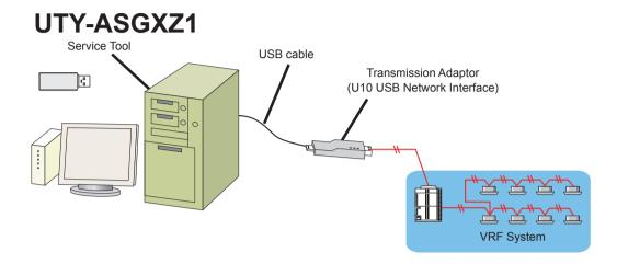
This transmission adaptor U10 USB Network Interface is connected using the USB port of a personal computer.
