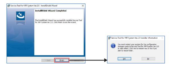
) After all the setup is completed, restart the Windows<sup>®</sup>.
