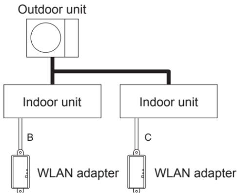
A, B, and C: Adapter cable attached to this product.
