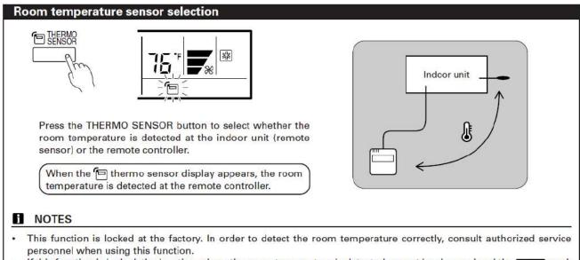
• If this function is locked, the location where the room temperature is detected cannot be changed and the o-m mark flashes when the THERMO SENSOR button is pushed.
