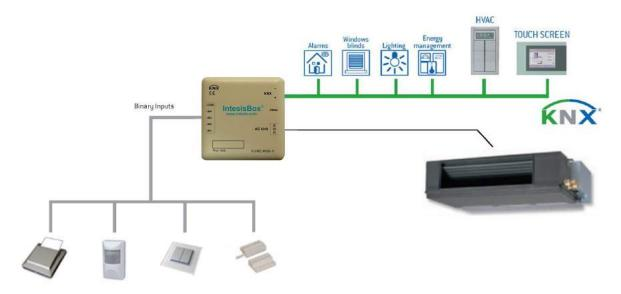
FJ-RC-KNX-1i allows a complete and natural integration of Fujitsu air conditioners with KNX control systems.
